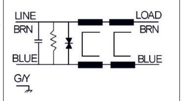
Operating Voltage = 100 VDC Operating Current (Max) = 20 Amp @ 50oC 15 Amp @ 70oC
